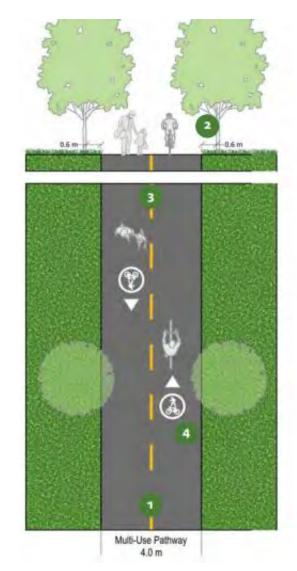
may change depending on the intended user groups, with asphalt surfaces being appropriate where pedestrians and/or cyclists are the primary user group, or crushed aggregate and wood chip surfaces if equestrian users are prevalent. Depending on surface materials these pathways could not be appropriate for people of all ages and abilities.
